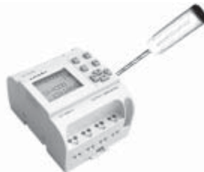
Fig. 2.1 Remove LCD panel as instructed
