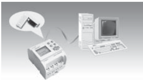
Fig. 4 . 24. FAB Communication Connection Frame
